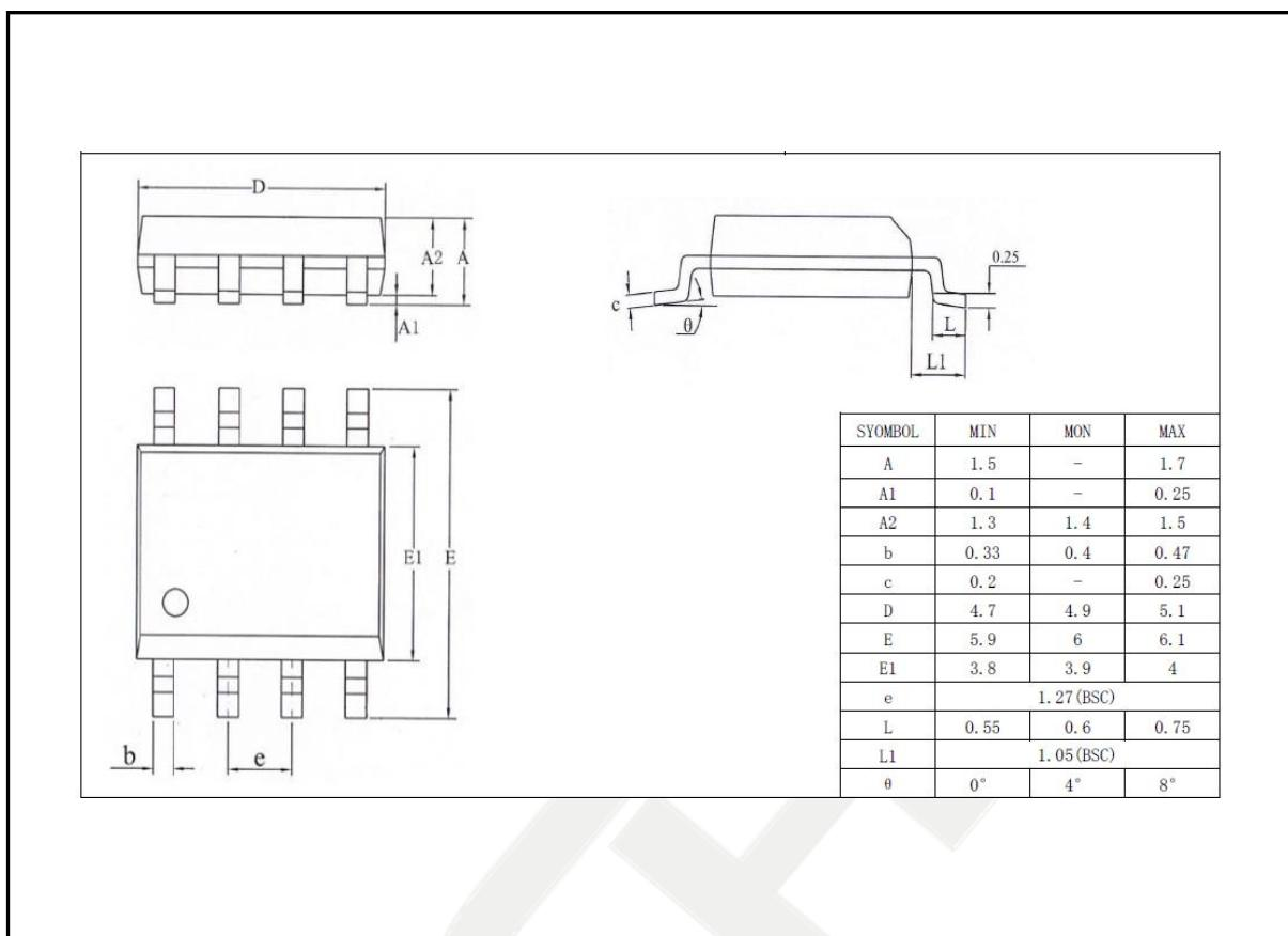
**Figure 12 SOT23-8L Mechanical Data and Package Dimensions**
